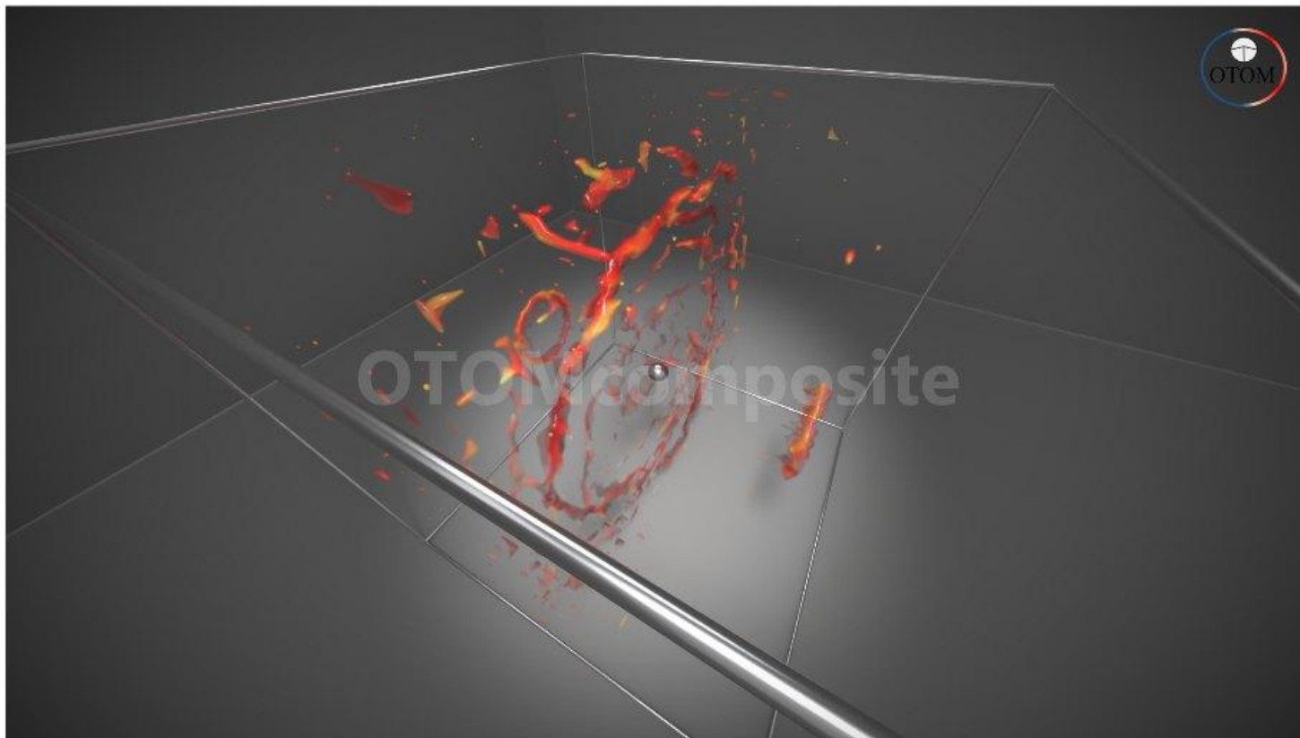
Q-criterion vortex-core surfaces (Jet colours). Blender (Cycles) render of the recorded run.
